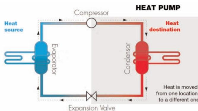
Now the important point of note here is that the heat 'source' and the heat 'destination' are separate, for instance in an air source heat pump you are removing heat from the external air to heat an internal space, in a bore hole you are removing heat from the ground water to heat the internal space. The important thing is that the source and the destination are not in the same space and the overall function is to move heat.
