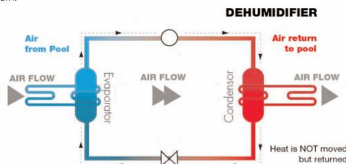
In this function there is no separation between the 'source' of heat and the 'destination'. In this application you cool the pool hall air down and then heat the same air back up again. This is why the swimming pool refrigerant-based air recirculation systems are dehumidifiers and not heat pumps.
