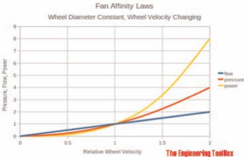
You can see the dramatic effect reducing the air volume can have on the power consumption of the motor. If we reduce the air volume down to 50%, we would reduce the power consumption to only 12.5% of the maximum. To put that into figures, a unit that takes 2.5 kW on maximum load would be reduced to 0.3 kW if the unit were running at half speed.
