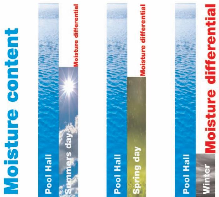
Throughout the year the fresh air has lower moisture content than the air inside the pool hall. By introducing fresh air in any of these conditions it will lower the moisture content of the pool hall and thus the relative humidity within the pool hall.
