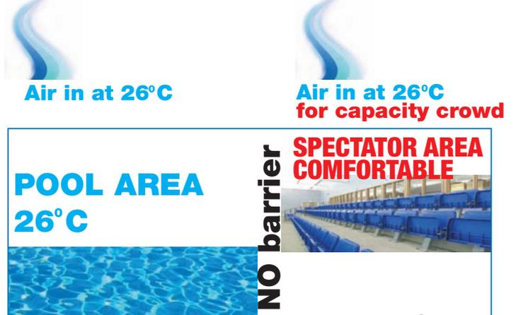
It's an extremely elegant, effective solution and most importantly it's cost-effective. Running costs are controlled to be as low as possible by only using one air handling unit, whilst providing conditions that are comfortable for both bather and spectator when appropriate.
